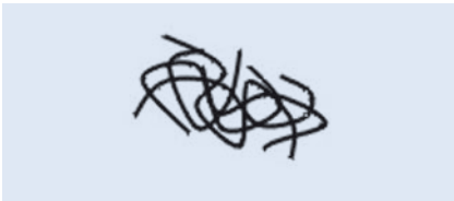
Polymer clumping in the case of thermoplastics (schematic diagram)
