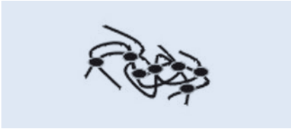
Structure of thermosets (schematic diagram)
