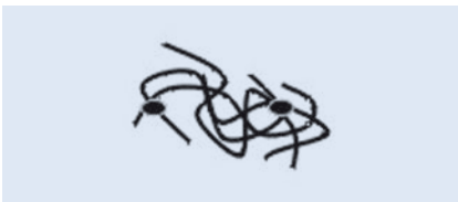
Structure of elastomers (schematic diagram)
